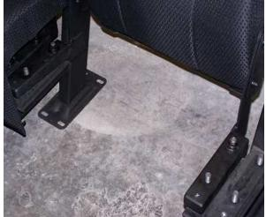
Each back bracket has 2 pre drilled holes that fit right onto the 2 bolts of each leg. You will need to install the back nuts and washers on your left and right legs at this time. Once you have tightened down these nuts and washers you are ready to mount your seat.
