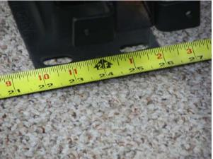
When mounting your Standards (legs) on 24 inch centers in the area that you have chosen for your chair(s), If anchoring to concrete we suggest using Quick Bolts, you can get these at most hardware stores. If mounting to wood use 1 3/4 3/8 lag bolts to mount legs, once this step is done your ready to mount your backs.
