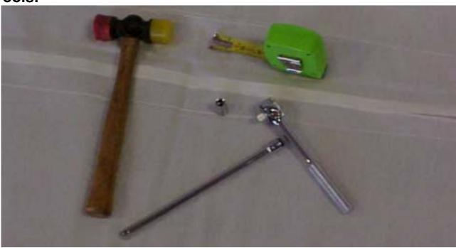
Tools that you will need are: Hammer, Measuring tape, 10 mm Socket, Extension to socket.
