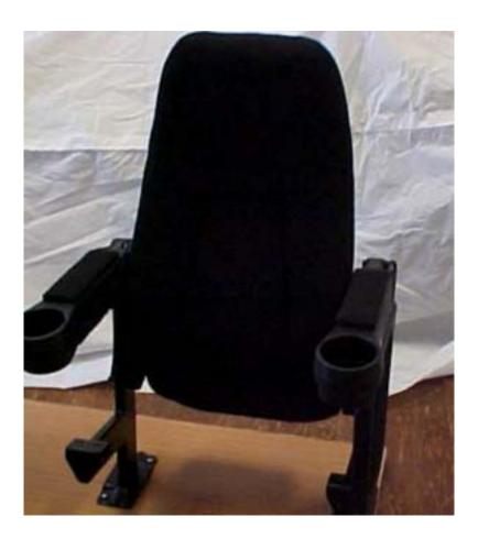
The Seat back must be level, not cockeyed. Now bring the chair back to a straight up and down position, (Do this by pushing the chairs back away from your body) while you are pressing firmly down on the back. If you have pushed firmly enough the pins on the standard will click into the slotted holes on the side of the back. It will now be in the upright position.
